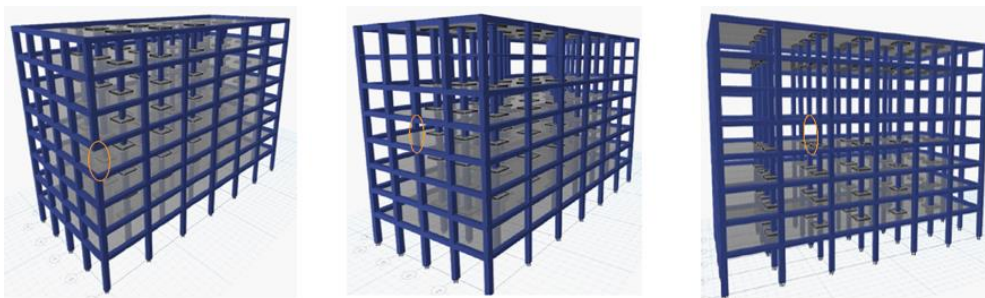
Fig. 5. Details of the model with static column removal for flat slab with drop panel and edge beams building
